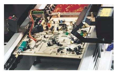
High measurement speed, two-channel measurements and remote-control capability via the IEC/IEEE bus are a must in production systems. The long calibration intervals of the R&S UPL make for high availability and reduce costs.
