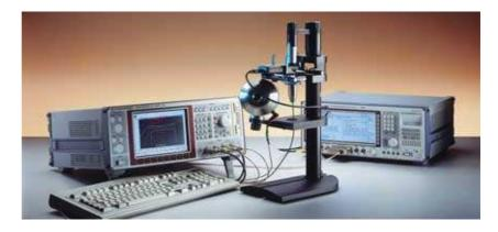
acteristics of commercial mobiles. A highly accurate test method is also required for quality assurance and sampling inspection in the production of mobile phones.
